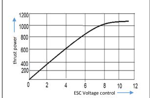
Fig. 2.3 .The thrust power and the supply is shown in the form of graph
