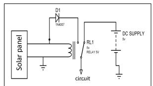
Fig. 2.5 Smart Saver circuit – useful for saving battery power during day time. Specially designed for Arduino
