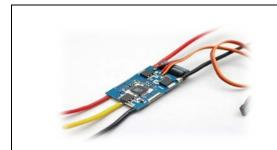
Fig. 2.2 Circuit board of ESC rating of 40 Amps.
